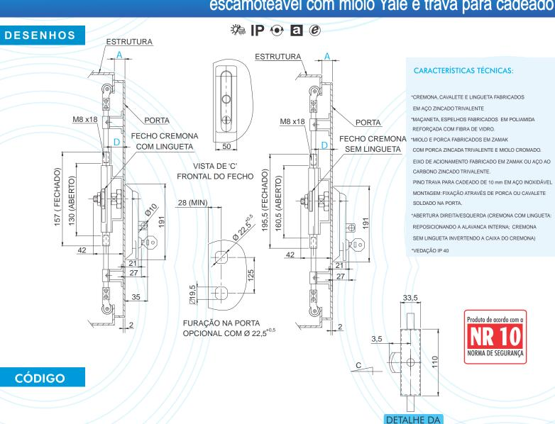
**PROFUNDIDADE** DA ABA DOBRADA **MIOLO** (D) (A) YALE **COM LINGUETA** 11,0 mm FC 51512 20 mm FC 51612 17,5 mm 26 mm **SEM LINGUETA** FC 51522 11,0 mm 17,5 mm FC 52622 26 mm
